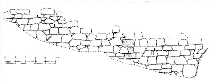
Fig. 3. The outer wall face of the southern spur wall with the masonry chain marked.
